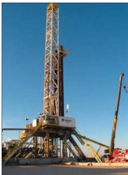
Nabors F-16 is a new 1,500-hp, Chinese-built PACE rig currently drilling in Libya for Occidental Petroleum Corp. (Fig. 3; photo from Nabors Industries Ltd.).
