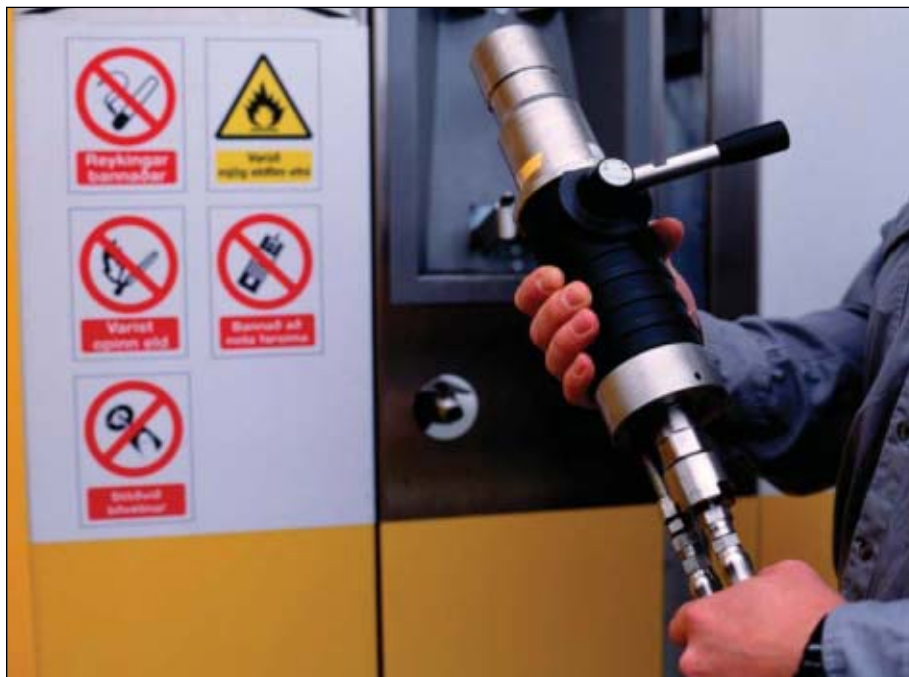
Shell Hydrogen provides a hydrogen-fuel dispenser to refuel fuel-cell buses at a station in Reykjavik, Iceland. Photo from Shell Hydrogen.
